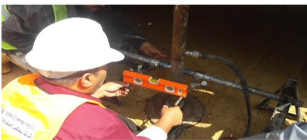
Plate Load Test on Soil Replacement
