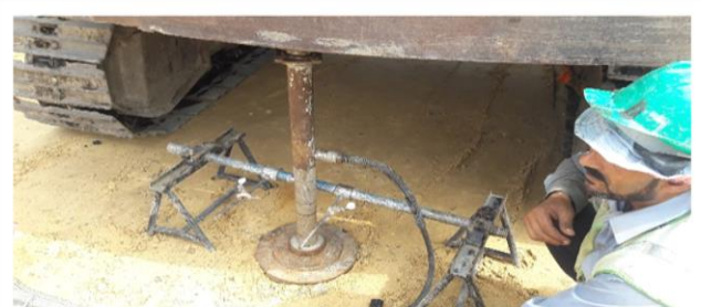
Plate Load Test on Soil Replacement
