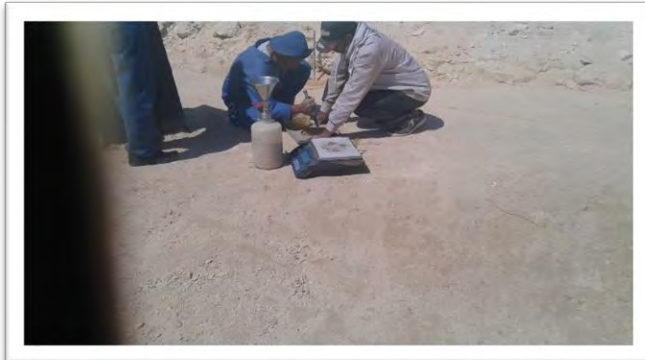
Test for soil compaction
