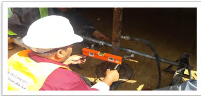
Plate Load Test on Soil Replacement
