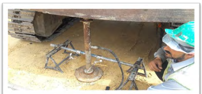
Plate Load Test on Soil Replacement
