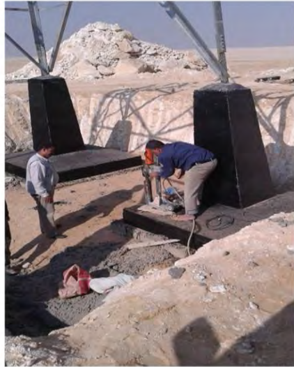
Core Test for Quality control
