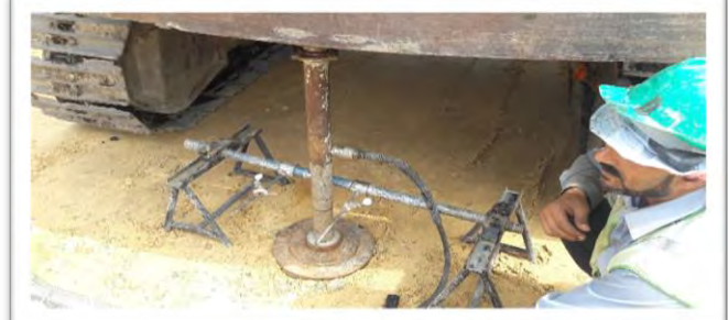
Plate Load Test on Soil Replacement
