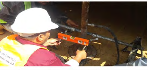
Plate Load Test on Soil Replacement
