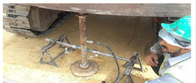
Plate Load Test on Soil Replacement
